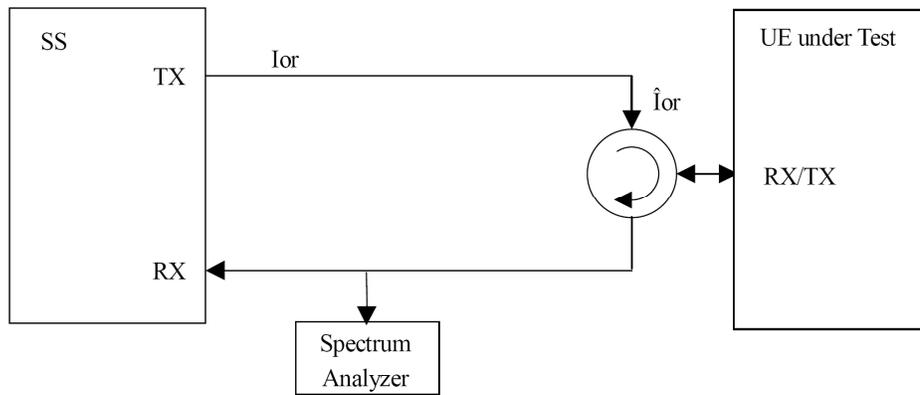
Figure C.6 - Connection for Spurious Emission Test
