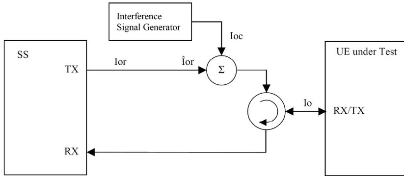
Figure C.2 - Connection for RX Test with Interference
