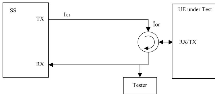
**Figure C.1 - Connection for Basic TX Test**
