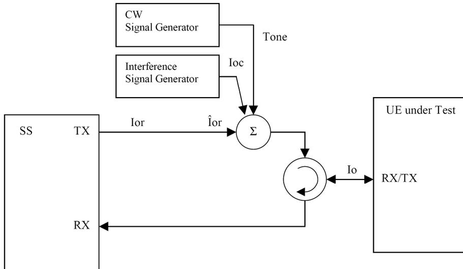
Figure C.5 - Connection for RX Test with both Interference and additional CW
