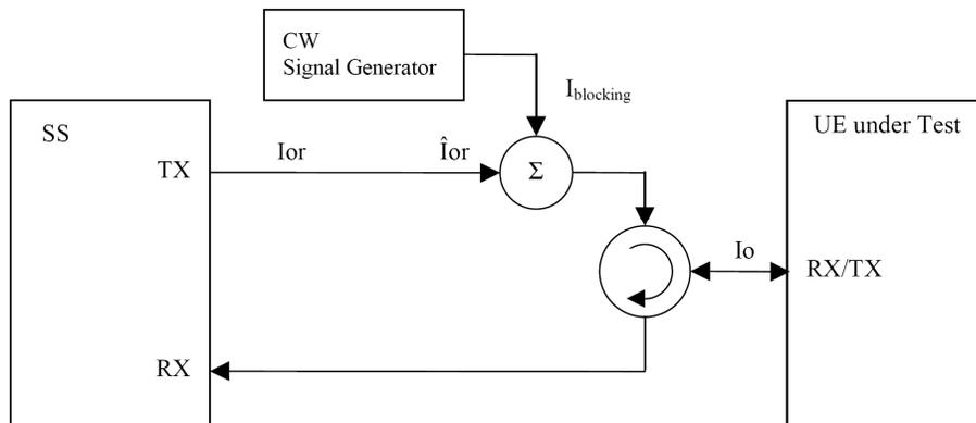
Figure C.4 - Connection for RX Test with additional CW
