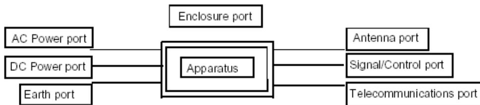
**Figure 1 - Examples of ports**
