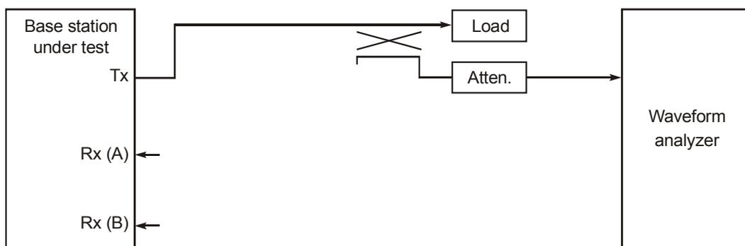
**Figure 5 - Functional Setup for Waveform Quality Test**
