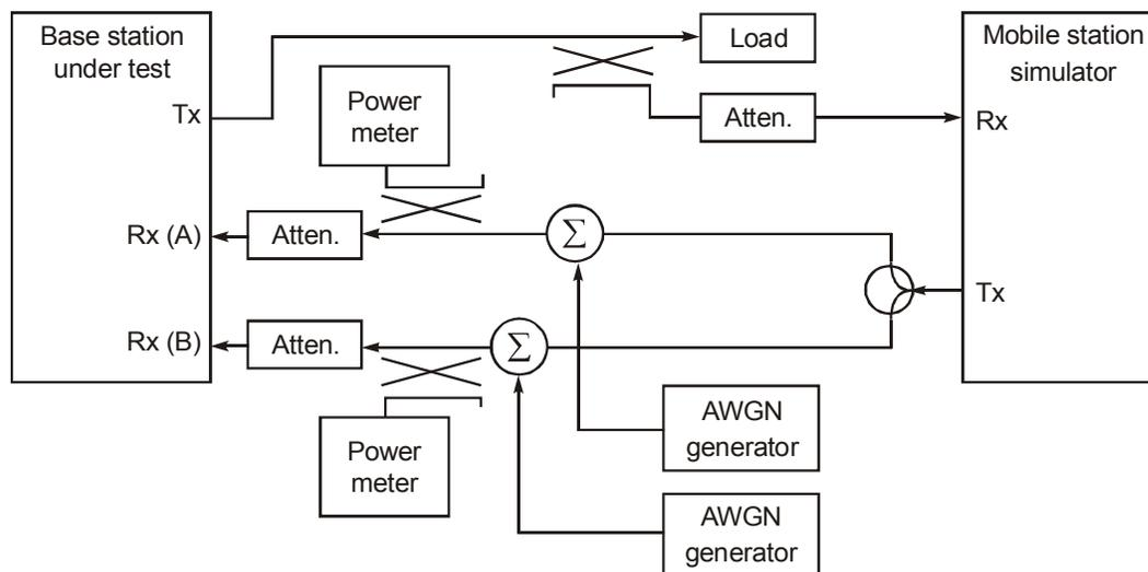
Figure 2 - Functional Setup for Base Station Sensivity Tests
