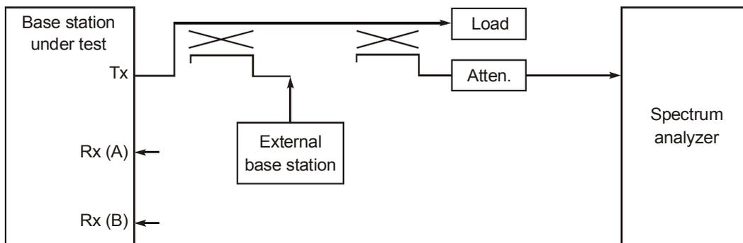
**Figure 8 - Functional Setup for Inter-Base Station Intermodulation Tests**
