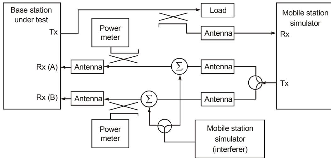
Figure 9 - Functional Setup for Base Station ACS Tests
