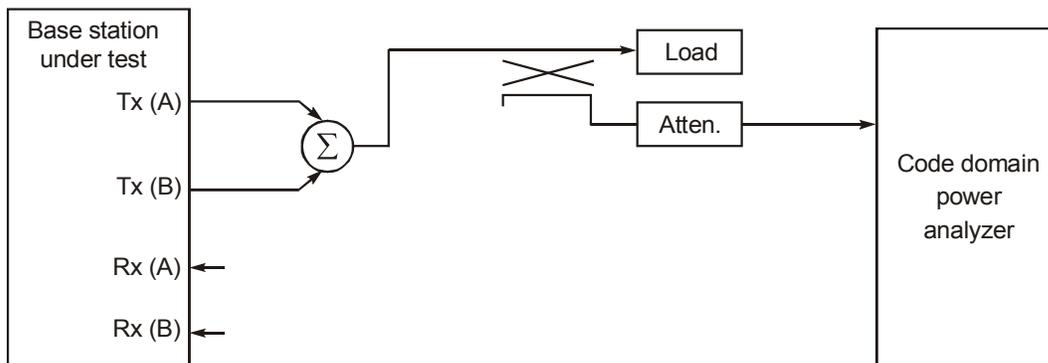
**Figure 7- Functional Setup for Code Domain Power Test for Transmit Diversity Configuration**
