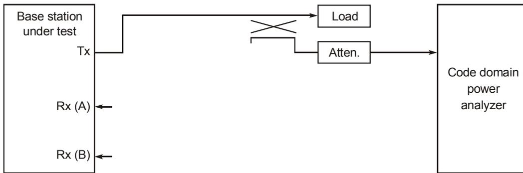
**Figure 6 - Functional Setup for Code Domain Power Test for Non-transmit Diversity Configuration**
