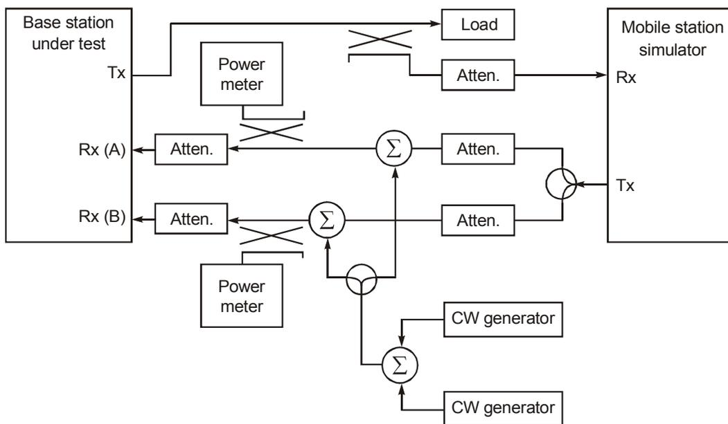
**Figure 4 - Functional Setup for Base Station Intermodulation Spurious Response Tests**
