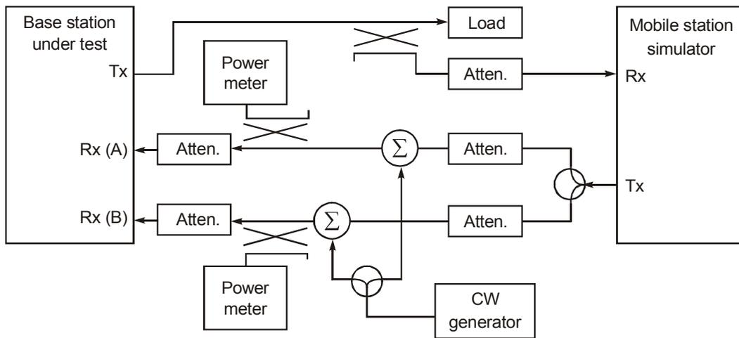
**Figure 3 - Functional Setup for Base Station Desensitization Tests**
