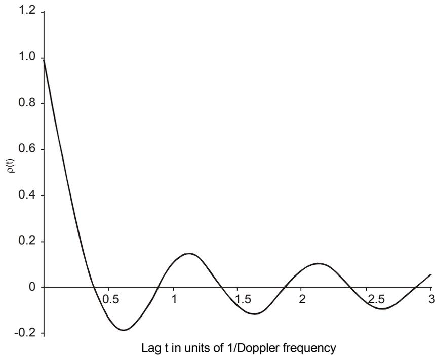
**Figure 1 - Autocorrelation Coefficient of the Phase**
