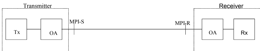
Figure 2 - Standard configuration of optical interface for systems using optical amplifier
