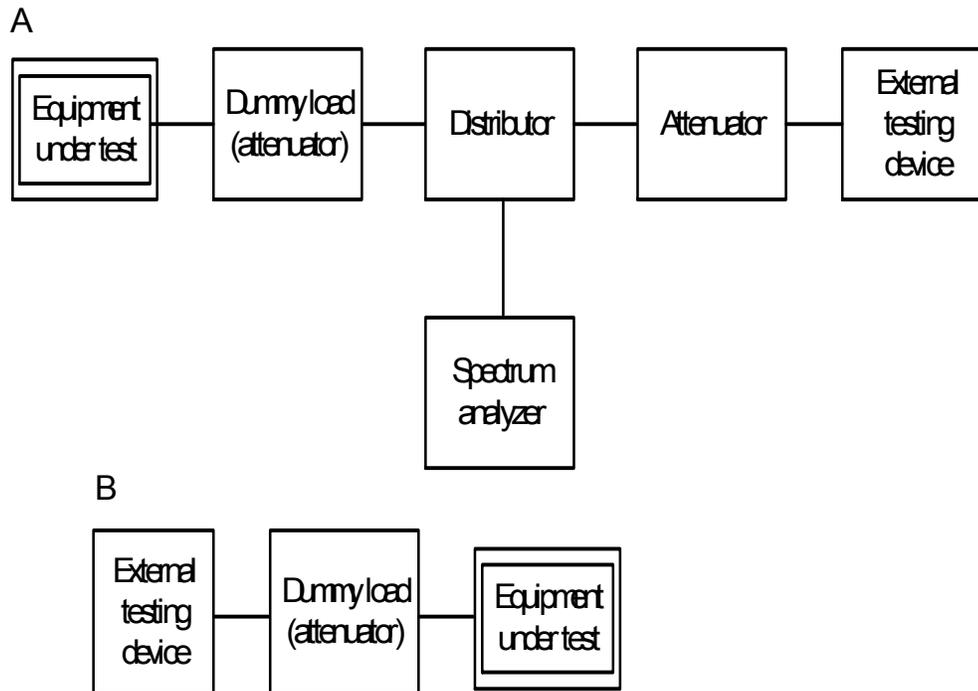
**Figure 33- Measuring system block diagram for transmission of calling identification code**
