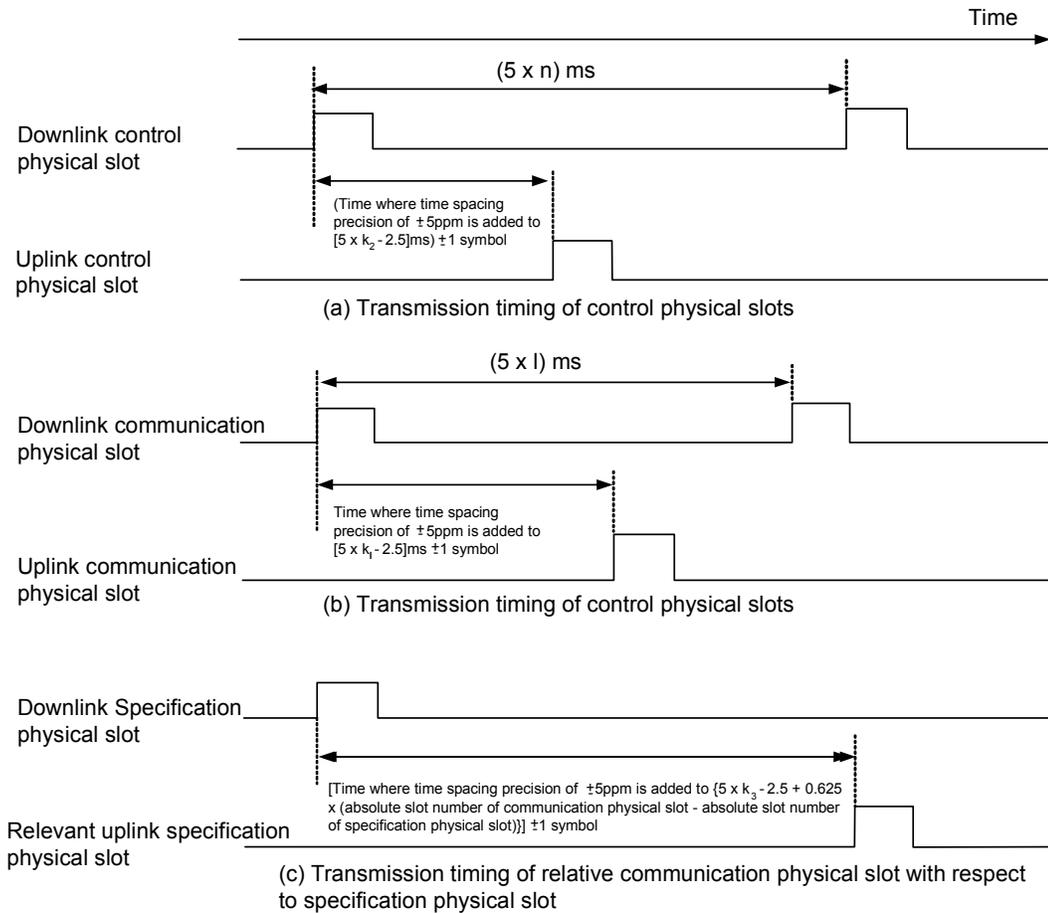
(Note) Figure (a), (b) and (c) show timing at the PS antenna terminal when wave propagation delay is not included
