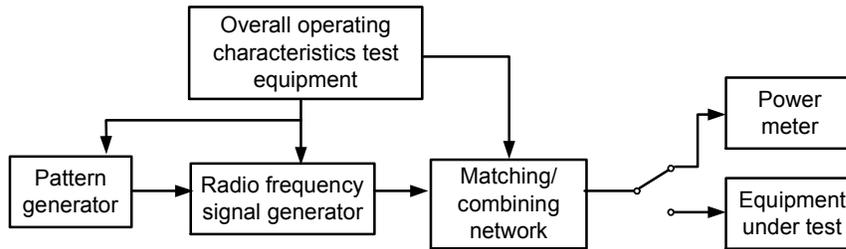
**Figure 26 - Measurement diagram for carrier sensing**
