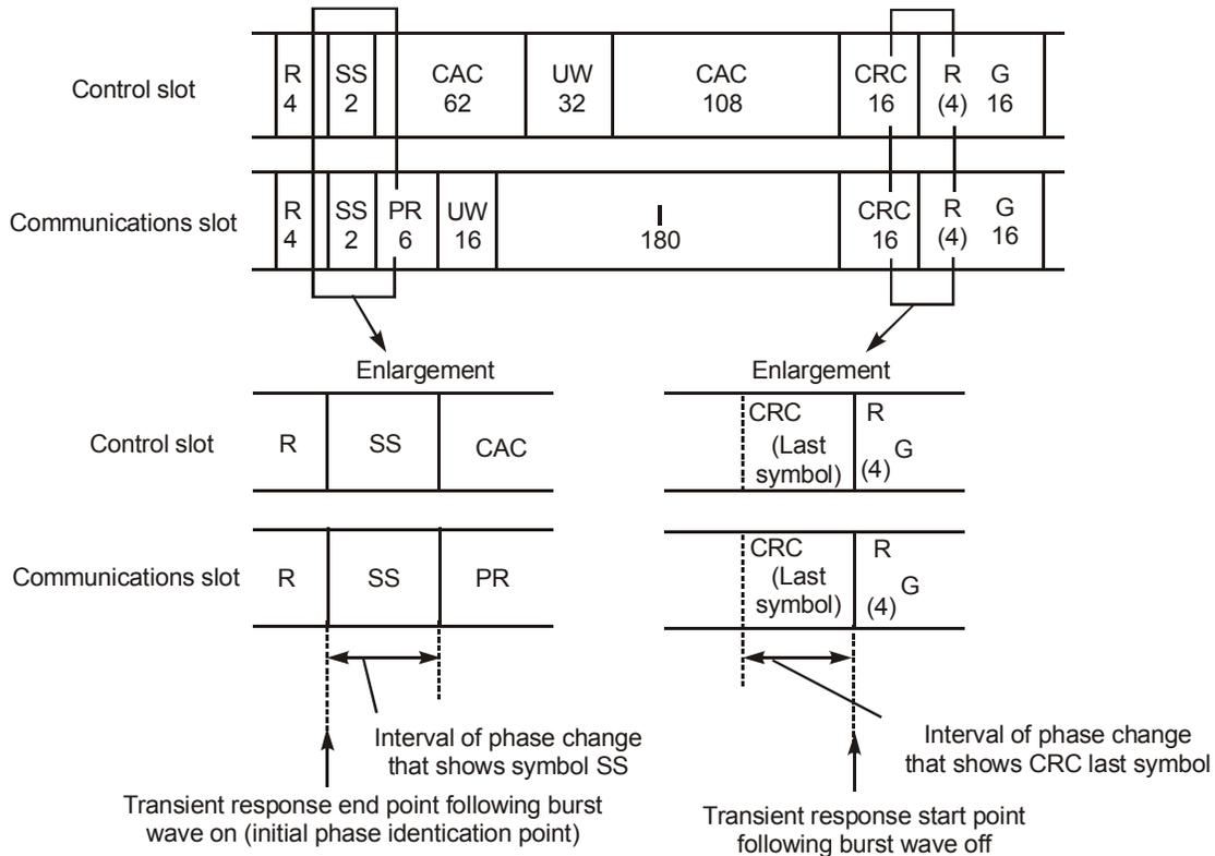
**Figure 4: Relationship between slot structure and burst wave on/off control**
