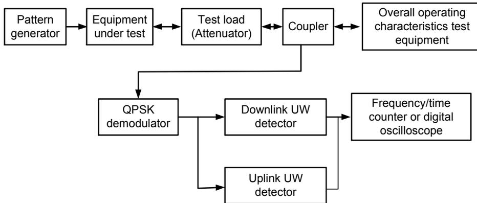
**Figure 18 - Measurement system diagram for Transmission timing a**
