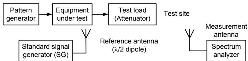
**Figure 16 - Measurement diagram for Cabinet radiation**
