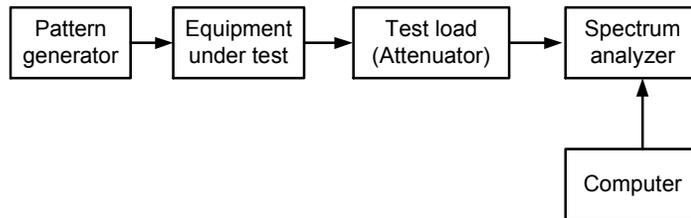
**Figure 15 - Measurement of Adjacent channel leakage power**
