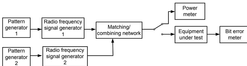
**Figure 22 - Measurement system diagram for Adjacent channel selectivity**
