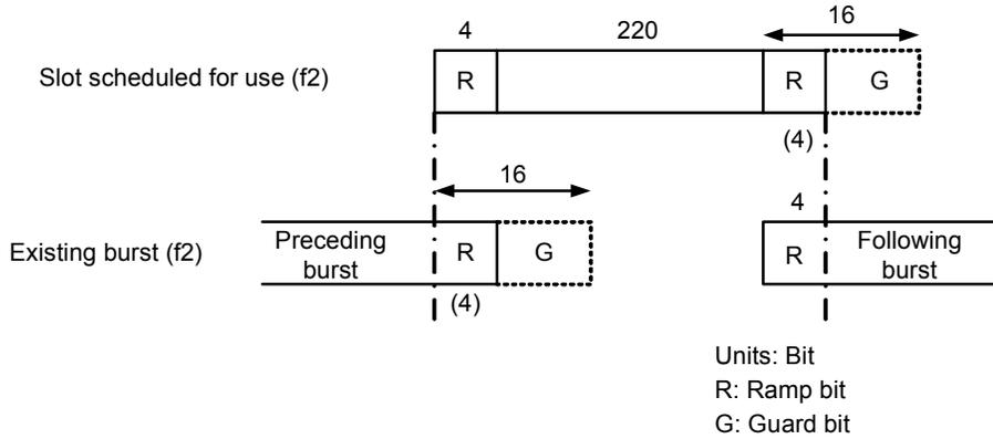
**Figure 1 - Carrier sensing method in PS side**
