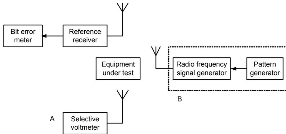
**Figure 31- Measurement Diagram for Sensitivity (test site measurement)**
