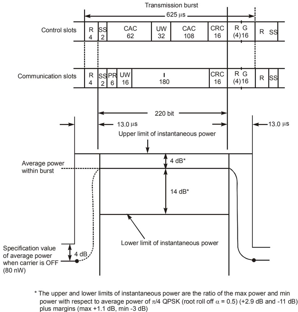
**Figure 3 - Standards of transmission power time response**
