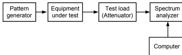
**Figure 9 - Measurement diagram of occupied bandwidth**
