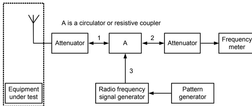
Figure 30 - Measurement system diagram in case of no transmission data input terminal
