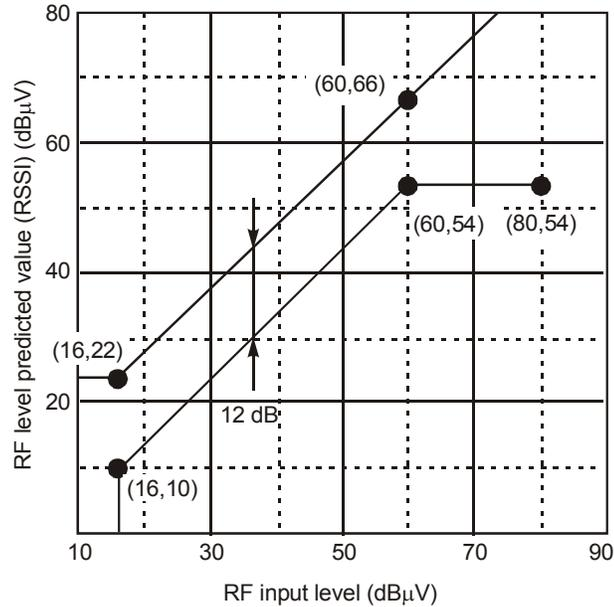
Figure 5 - RF input level indicator accuracy
