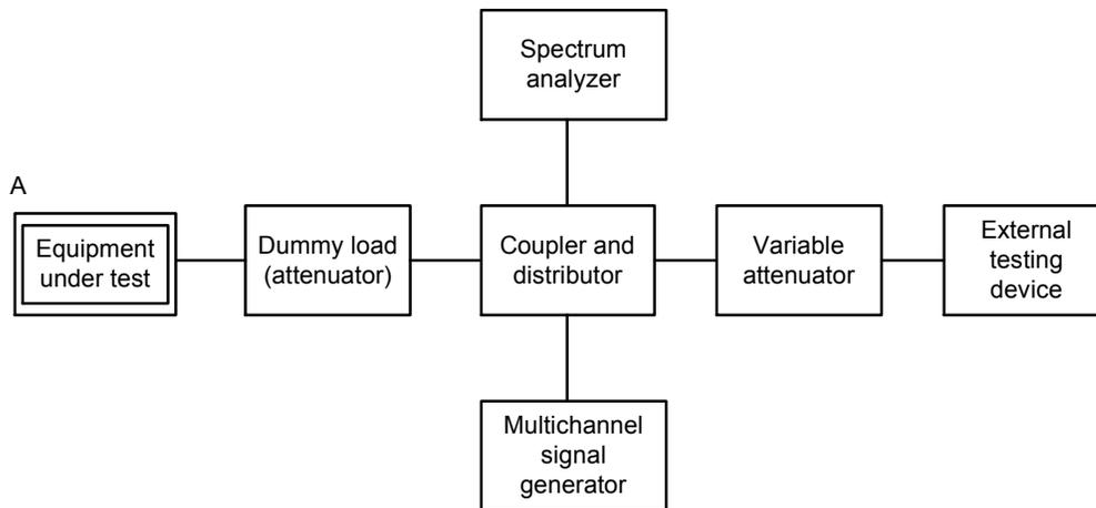
**Figure 34 - Measuring system block diagram for control channel**
