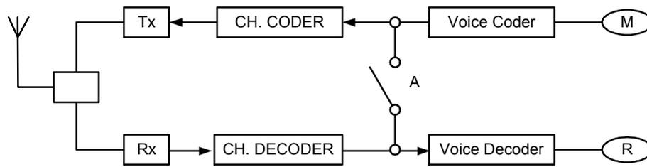
Figure 29 - Measurement system diagram
