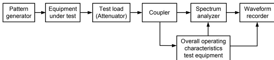
**Figure 13 - Measurement diagram of transient characteristics of burst transmission**
