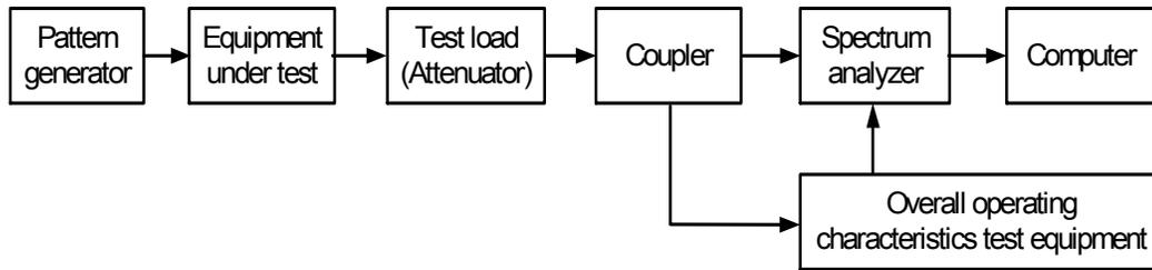
**Figure 12 - Measurement diagram of carrier offtime leakage power**
