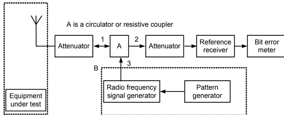
**Figure 32 - Measurement diagram when there is no data output terminal**
