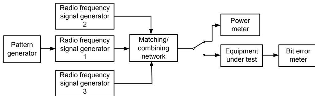
**Figure 23 - Measurement system diagram for Intermodulation characteristics**
