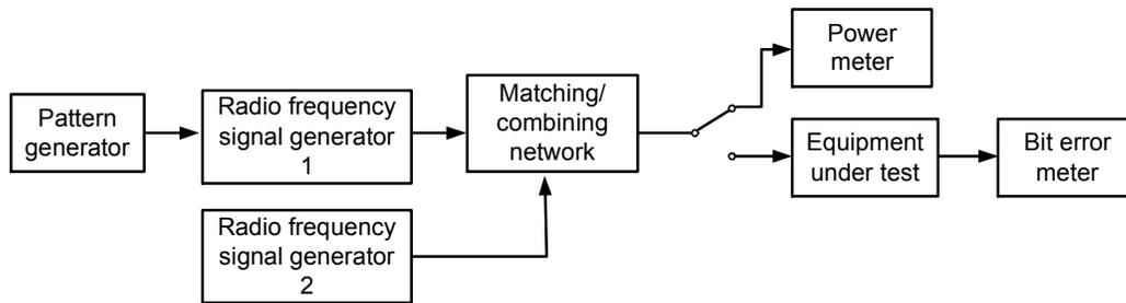
**Figure 24 - Measurement system diagram for spurious response immunity**
