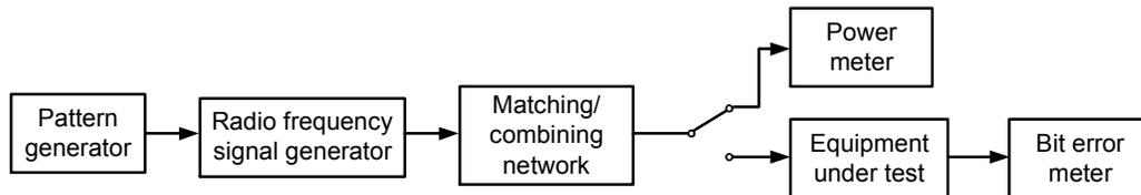
**Figure 21 - Measurement system diagram for Sensitivity**
